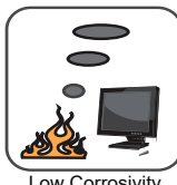
Low Corrosivity IEC60754-2 EN50267-2-2/3 NF C 32-074
