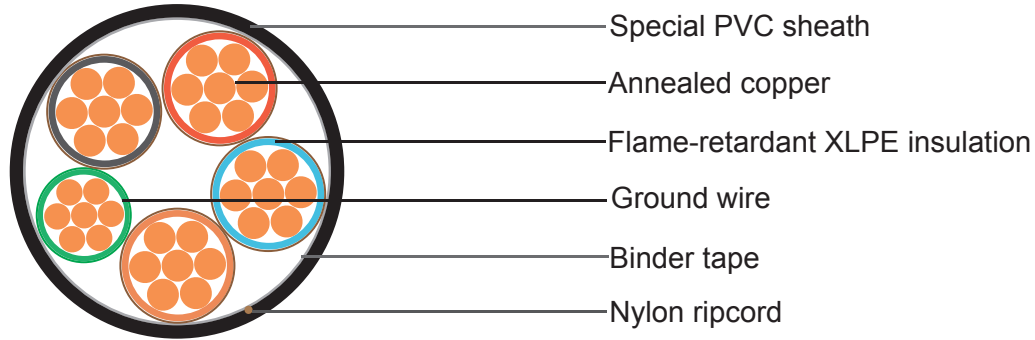
Unscreened XHHW-2 Cable with Ground Wire
