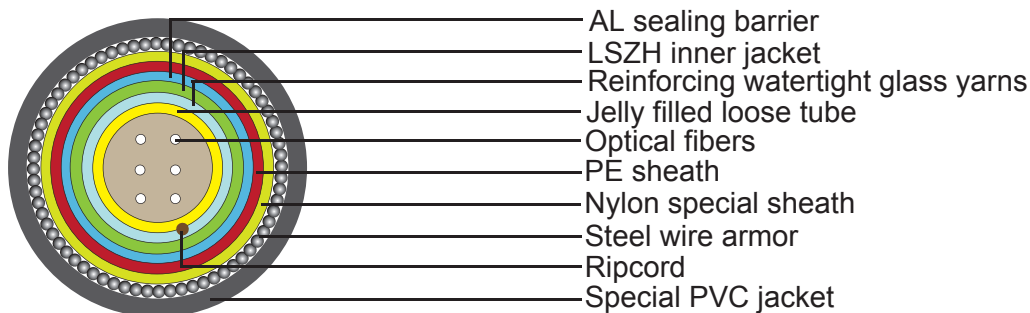
Steel Wire Armored Optical Fiber Cable with Special Sheath
