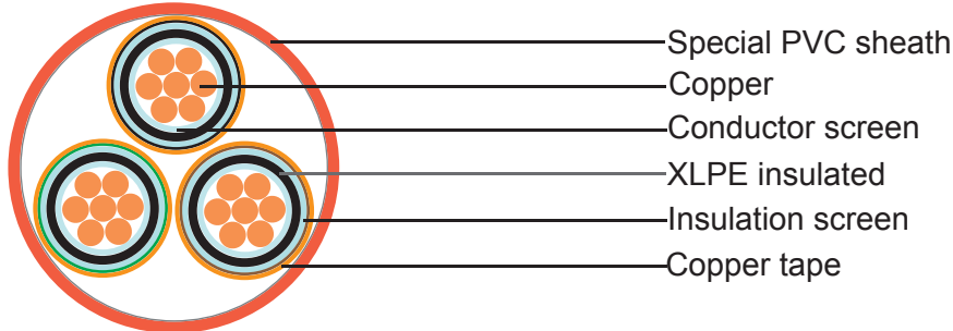
XLPE Insulated Cable to IEC 60502-2
