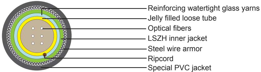
Steel Wire Armored Optical Fiber Cable
