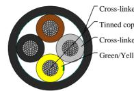
Cross-linked silicone jacket Tinned copper conductor Cross-linked silicone insulation Green/Yellow wire
