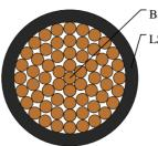
Bare copper conductor LSOH cross-link polyolefin insulation
