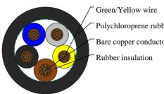
Polychloroprene rubber outer jacket Bare copper conductor
