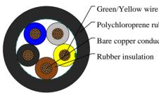
Polychloroprene rubber outer jacket Bare copper conductor
