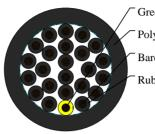
Green/Yellow wire Polychloroprene rubber outer jacket Bare copper conductor Rubber insulation
