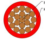
Bare copper conductor Rubber compound insulation
