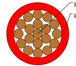
Bare copper conductor Rubber compound insulation
