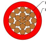
Bare copper conductor Rubber compound insulation
