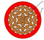
Bare copper conductor Rubber compound insulation
