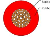
Bare copper conductor Rubber compound insulation
