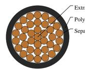
Extra fine bare copper conductor Polychloroprene rubber jacket Separator
