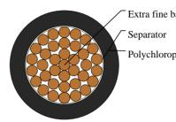
Extra fine bare copper conductor Separator Polychloroprene rubber jacket
