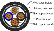
Flat steel wire with steel tape armour Thermoplastic compound filler Plain copper conductor
