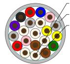
Plain copper conductor Halogen free outer jacket Halogen free insulation
