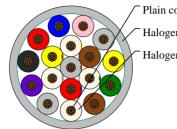
Plain copper conductor Halogen free outer jacket Halogen free insulation
