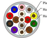
Plain copper conductor Halogen free outer jacket Halogen free insulation
