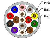
Plain copper conductor Halogen free outer jacket Halogen free insulation
