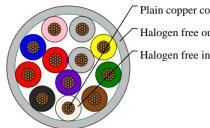
Plain copper conductor Halogen free outer jacket Halogen free insulation
