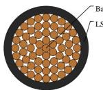
Bare copper conductor LSOH cross-link polyolefin insulation
