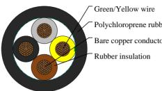
Polychloroprene rubber outer jacket Bare copper conductor
