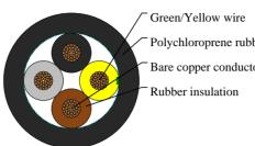
Polychloroprene rubber outer jacket Bare copper conductor
