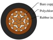
Bare copper conductor Polychloroprene rubber outer jacket Rubber insulation
