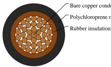
Bare copper conductor Polychloroprene rubber outer jacket
