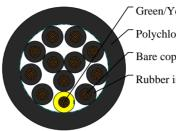
Green/Yellow wire Polychloroprene rubber outer jacket Bare copper conductor Rubber insulation
