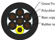
Green/Yellow wire Polychloroprene rubber outer jacket Bare copper conductor Rubber insulation
