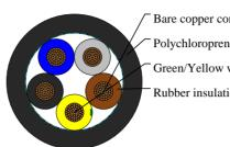
Bare copper conductor Polychloroprene rubber outer jacket Green/Yellow wire Rubber insulation
