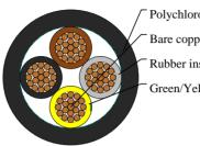
Polychloroprene rubber outer jacket Bare copper conductor Rubber insulation Green/Yellow wire
