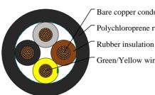
Bare copper conductor Polychloroprene rubber outer jacket Rubber insulation Green/Yellow wire
