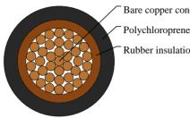
Bare copper conductor Polychloroprene rubber outer jacket Rubber insulation
