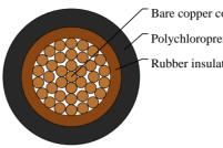
Bare copper conductor Polychloroprene rubber outer jacket Rubber insulation
