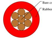
Bare copper conductor Rubber compound insulation
