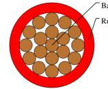
Bare copper conductor Rubber compound insulation
