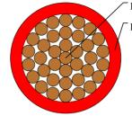
Bare copper conductor Rubber compound insulation
