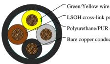
LSOH cross-link polyolefin insulation Polyurethane/PUR outer jacket Bare copper conductor
