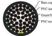
Bare copper conductor PVC outer jacket Green/Yellow wire PVC insulation
