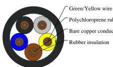
Polychloroprene rubber outer jacket Bare copper conductor
