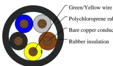
Polychloroprene rubber outer jacket Bare copper conductor
