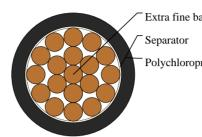
Extra fine bare copper conductor Separator Polychloroprene rubber jacket
