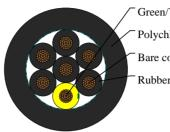
Green/Yellow wire Polychloroprene rubber outer jacket Bare copper conductor Rubber insulation
