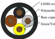
LSOH cross-link polyolefin insulation Polyurethane/PUR outer jacket Bare copper conductor Green/Yellow wire
