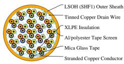
Tinned Copper Drain Wire XLPE Insulation Al/polyester Tape Screen Mica Glass Tape
