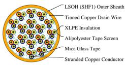
Tinned Copper Drain Wire XLPE Insulation Al/polyester Tape Screen Mica Glass Tape Stranded Copper Conductor
