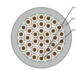
Stranded Copper Conductor LSOH (SHF1) Sheath XLPE Insulation
