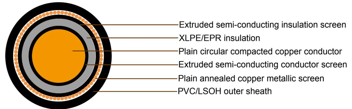
**CONDUCTOR:** Plain circular compacted copper to AS/NZS1125
