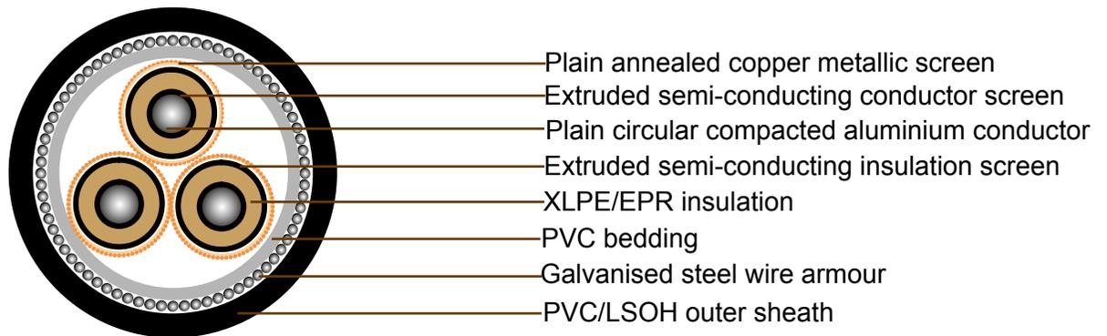
**CONDUCTOR:** Plain circular compacted aluminium to AS/NZS1125
