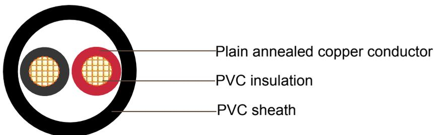
**Conductor:** Plain annealed copper.
