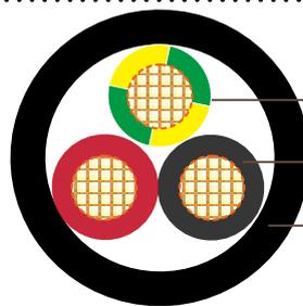
Plain annealed copper conductor
