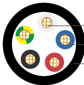
Plain annealed copper conductor
