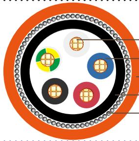
Plain annealed copper conductor
