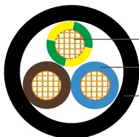
Annealed copper conductor
