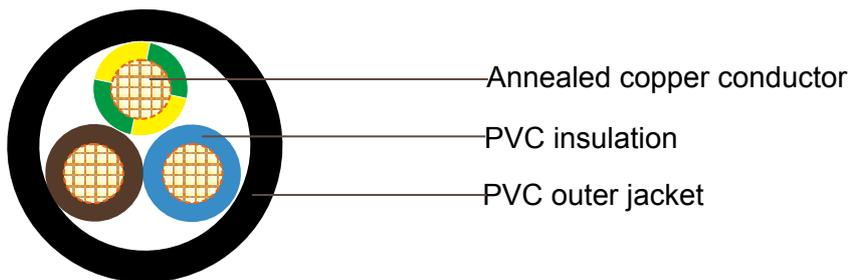
**Conductor:** Annealed copper conductor to AS/NZS 1125
