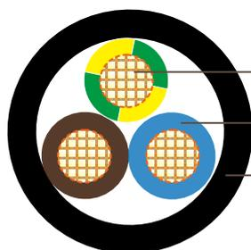
Annealed copper conductor
