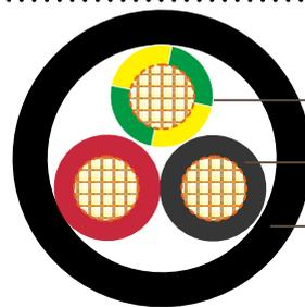
Plain annealed copper conductor
